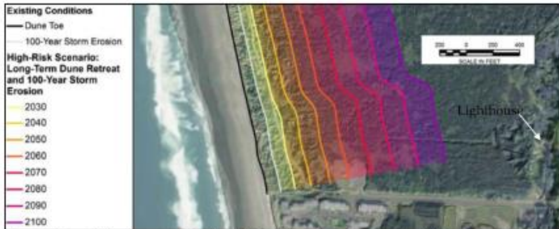
Figure 12. Projected shoreline retreat under the “high-risk” (i.e., 1% exceedance sea-level rise) scenario + 100-year storm event. Most of the land accreted since construction of the lighthouse in 1897/8. From Figure 17 of AECOM (2022a).
